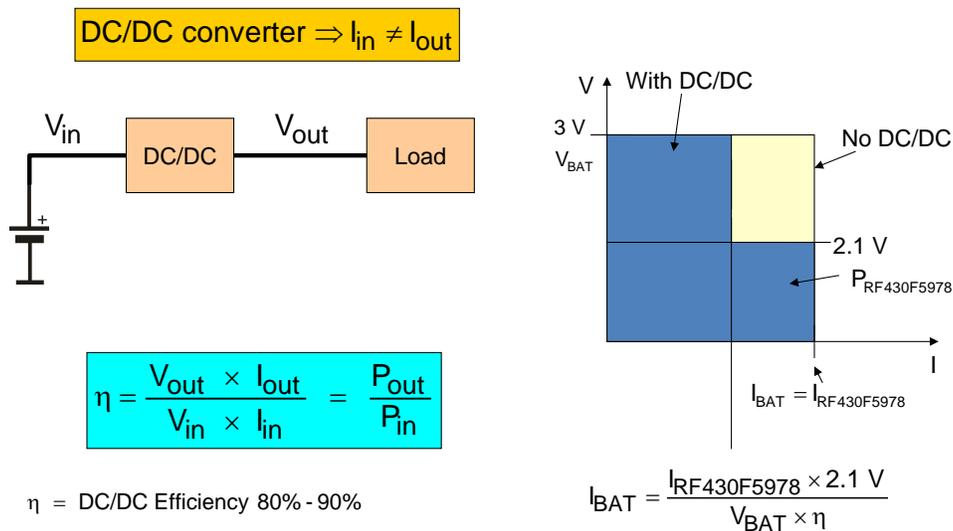
Figure 15. DC/DC Converter Scheme
