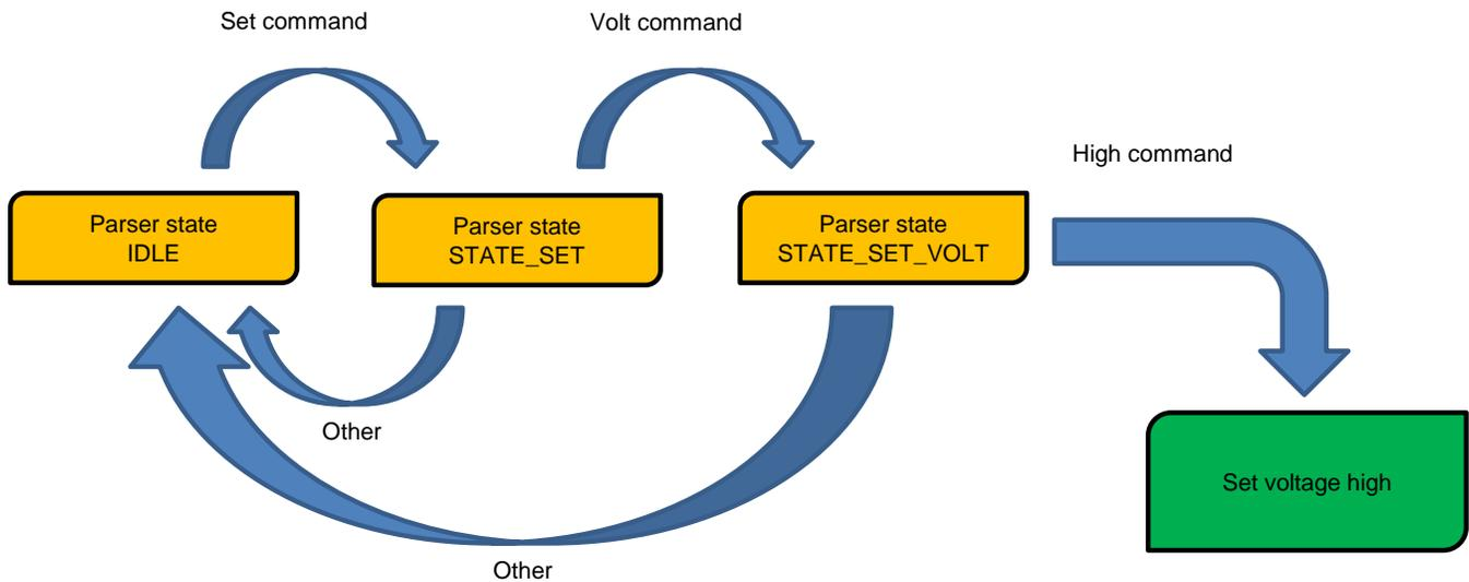
**Figure 9. Parser Example Flowchart**
