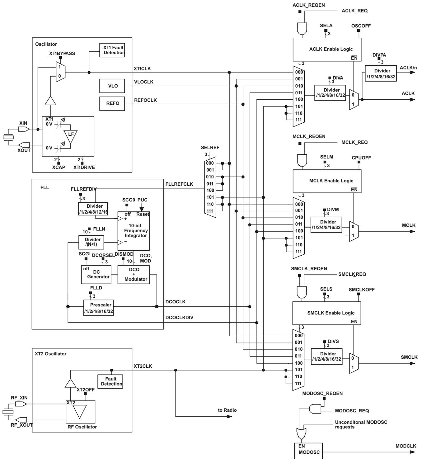
Figure 11. RF430F5978 Unified Clock System
