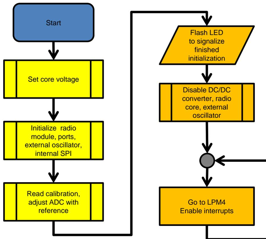
Figure 4. RF430F5978EVM Main Function Flowchart
