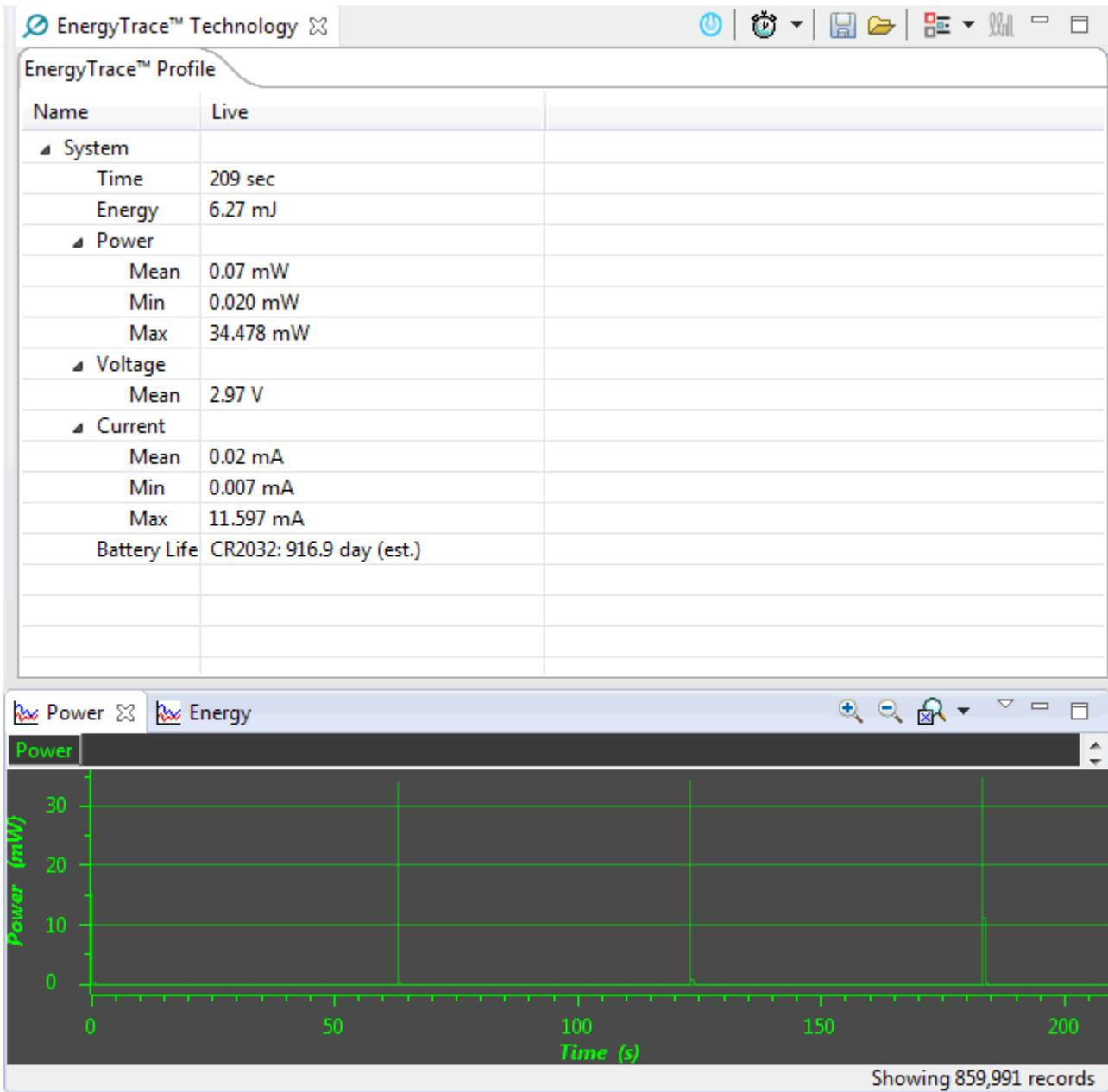
Figure 19. EnergyTrace™ Profile With Continuous Measurement
