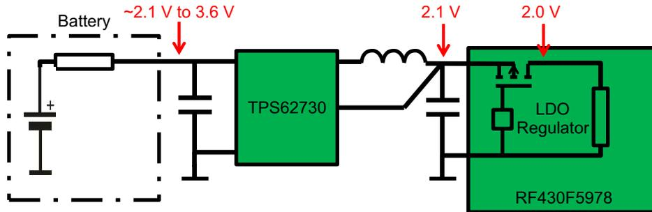
Figure 16. RF430F5978 TPS62730 Supply With Voltage Levels
