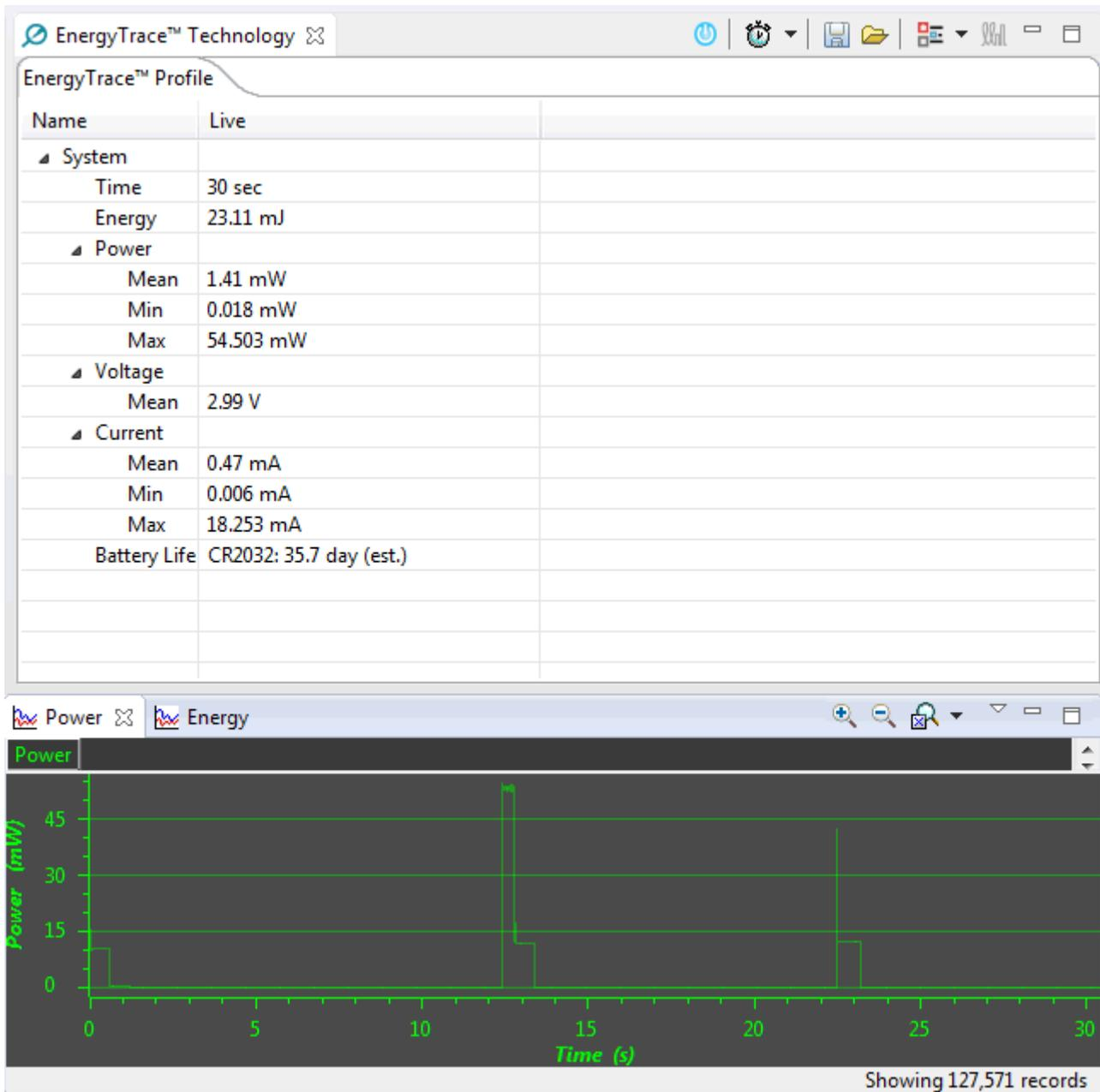
Figure 18. EnergyTrace™ Profile in RX Mode and TX Mode
