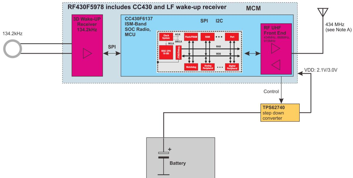
A 434-MHz worldwide frequency depends on the RF430F5978EVM RF filter and the selected UHF frequency condition. With different hardware, the kit can use the 315-, 868-, or 915-MHz bands.
