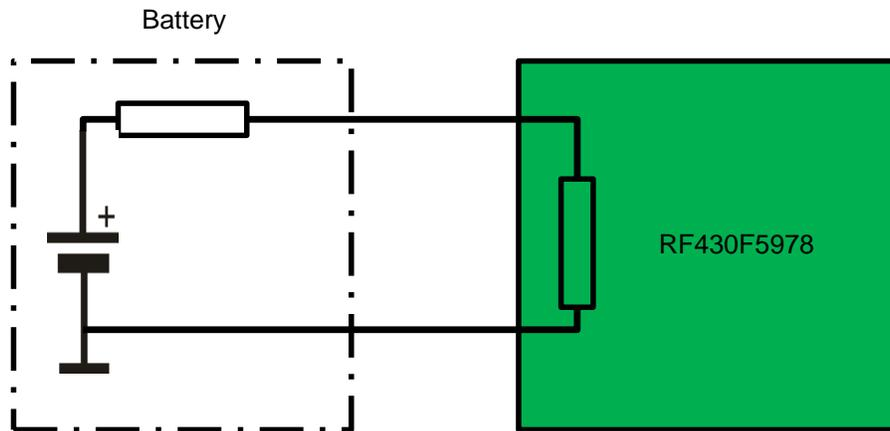
Figure 12. RF430F5978 Battery Supply
